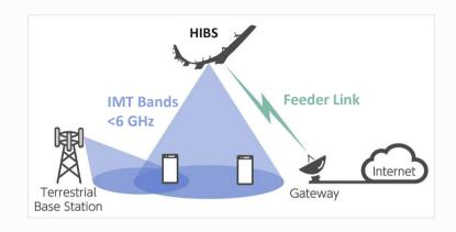
• HIBS are effectively a different type of base station – a super microcell that can expand coverage and complement existing macro, micro, and picocells used for urban and rural coverage.
